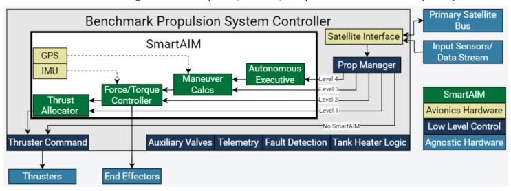
SmartAIM™ uses embedded sensors and an inner-control loop for thrusters and can incorporate additional effectors, sensors, and data input to eliminate positioning and propulsion command latency and generate more efficient and effective maneuvers than state-of-the-art operations.
