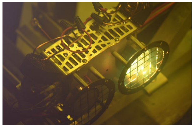
Figure 5. MPT2.0 Firing in VF-3 at NASA GRC
